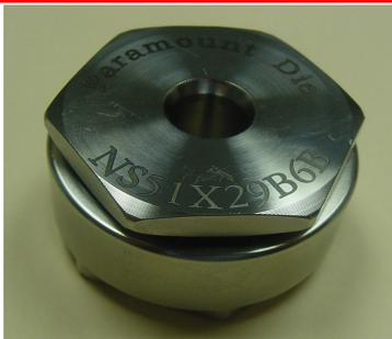
**c. ParaLoc Non-pressure Holders** - These holders come in standard die casing dimensions and include a locking cap to provide security against the insert backing out of the casing. As the precise taper tolerance on the insert generally provides adequate holding power, this option is only required in situations where excessive back tension may pull the insert out of the casing.
