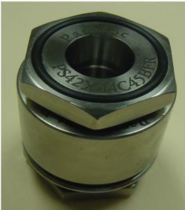
**a. ParaLoc Pressure Holders** - These holders have a base with a tapered bore for the drawing insert and includes space for a pressure insert in the cap. By pressurizing lubricant during wire drawing, the ParaLoc Pressure System enables optimal carry through and reduces drawing friction.
