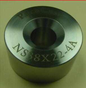
**b. ParaCase Holders** - These are the basic casings in standard dimensions with no locking cap. Inserts are simply tapped in and out of the casing. The precise taper tolerances on the insert and casing provide adequate holding power for most applications.
